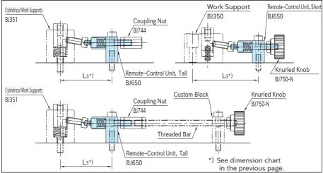
Suitable for controling work supports from a distance.
